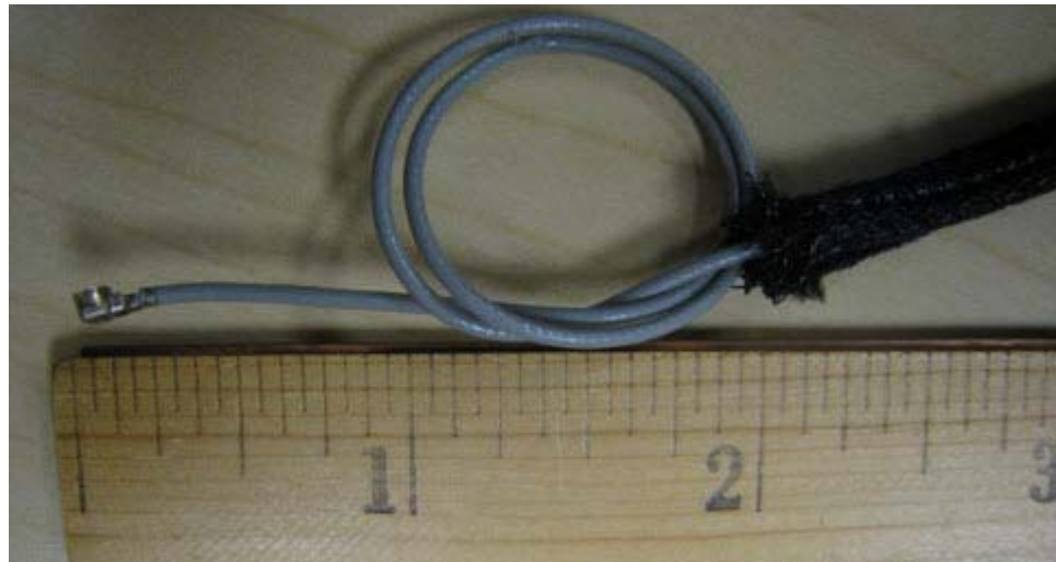
Figure B-10 cLLD coax cable coiled for installation
