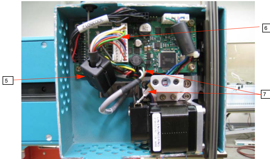
Figure 3-4 Attaching cables from the Y axis
