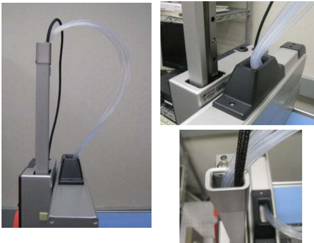
Figure 3-19 Proper routing of the tubing without tangles or rubbing
