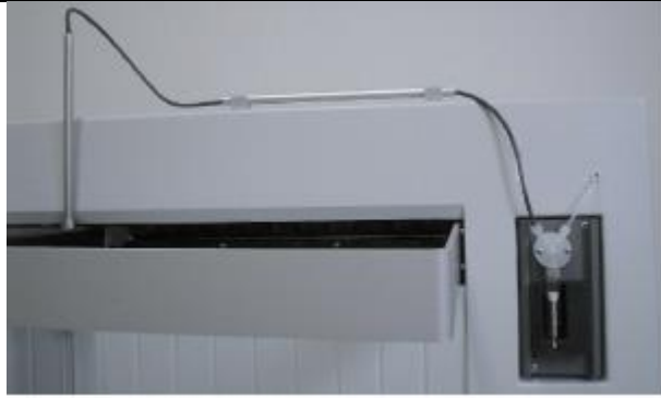
Figure 3: Installation of pipetting needle
